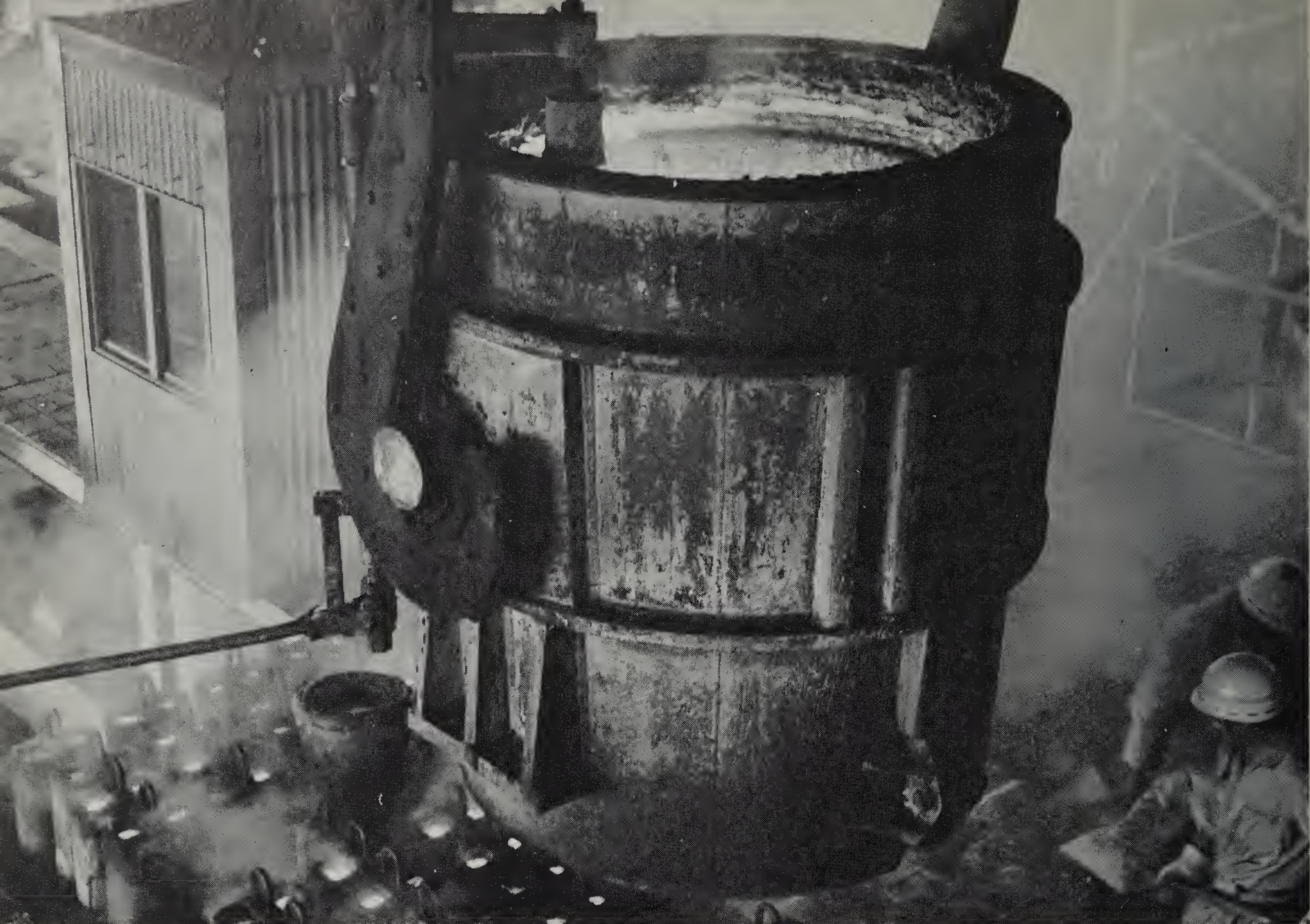
Steel ingots are being cast here at the new steel plant at Prai, Malaysia. The plant features import substitution, relying on local iron ore and rubber tree coke.
